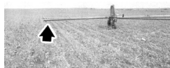
FIGURE 19. Sagging Boom End.
