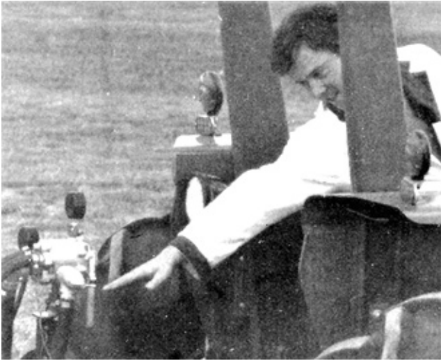
FIGURE 15. Controls Difficult to Reach from Tractor Seat.
