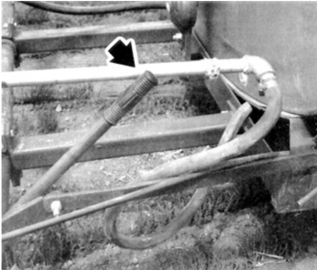
FIGURE 20. Interference Between Boom Adjusting Handle and Right Boom in Transport.
