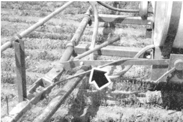
FIGURE 16. Interference Between Radius Brace and Boom Adjusting Linkage.
