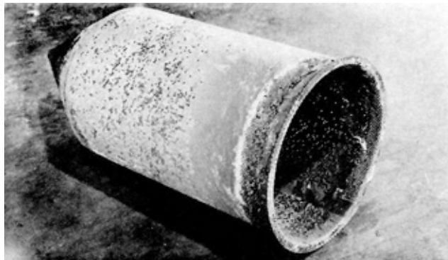
FIGURE 14. Separator Cyclone Screen Plugged with Fertilizer.
