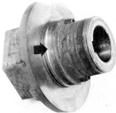
FIGURE 16. Worn Rotary Air Lock Hub.
