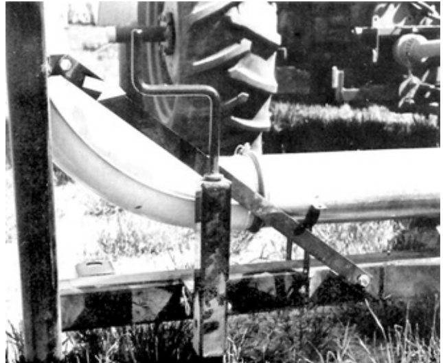
FIGURE 8. Interference between Jack Handle and Discharge Cyclone Support Bracket.
