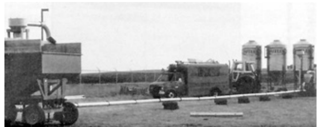
FIGURE 11. Increased Discharge Pipe Length.
