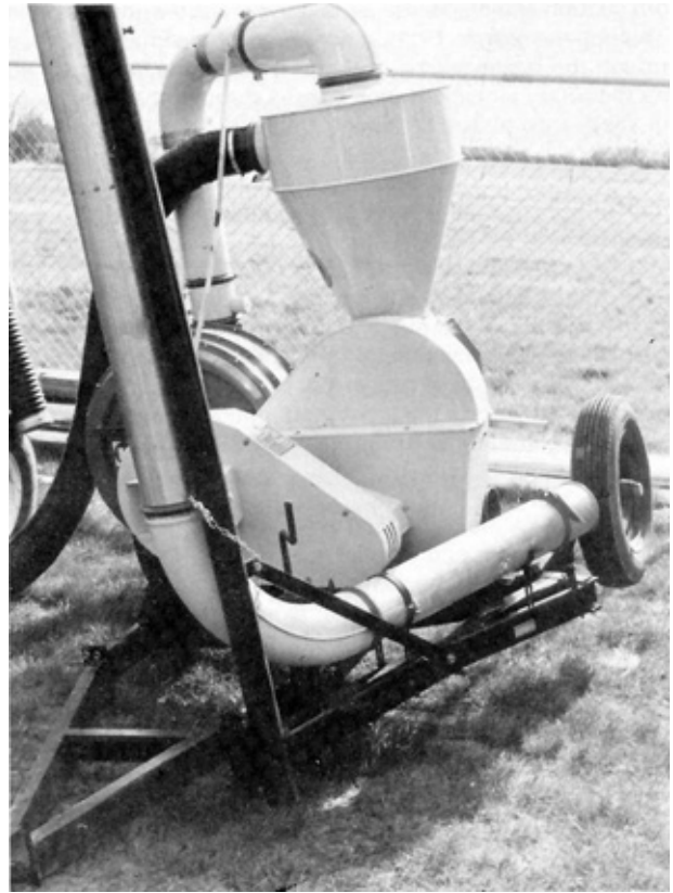
FIGURE 7. Unstable Transport Position.
