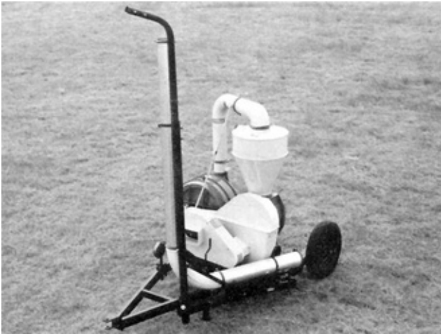
FIGURE 5. Transport Position with Discharge Cyclone Removed.
