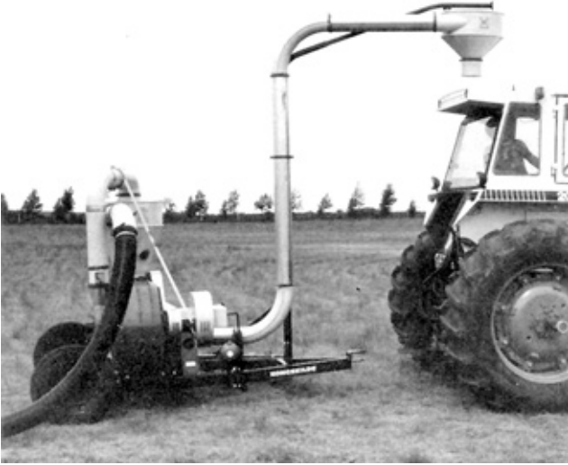
FIGURE 4. Limited Clearance in Transport Position between Discharge Cyclone and Tractor Cab.
