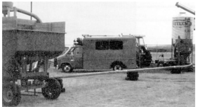
FIGURE 10. Increased Discharge Pipe Length.
