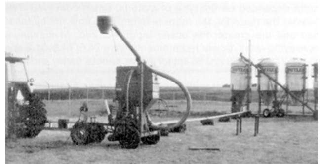
FIGURE 9. Increased Intake Pipe Length.
