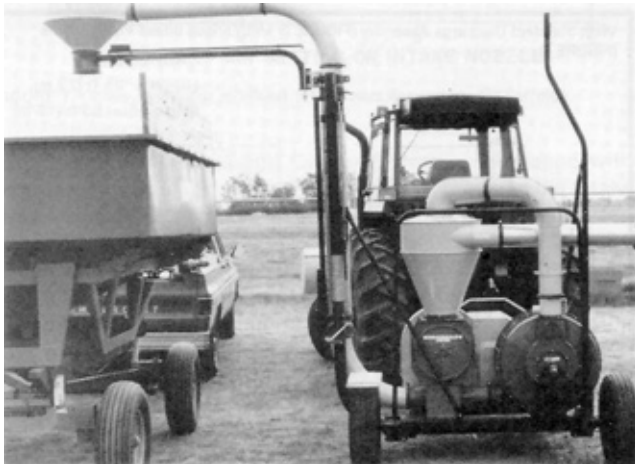
FIGURE 3. Intake Nozzle: (1) Adjustable Sleeve.
