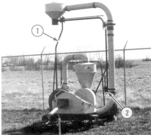
FIGURE 5. Kongskilde SUC 500 TR2 in Transport Position: (1) Support Bar, (2) Jack Assembly.
