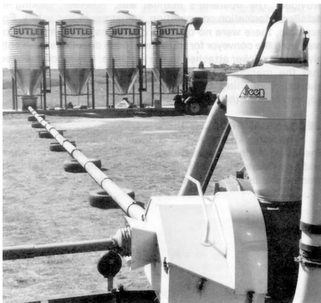
FIGURE 8. Increased Intake Pipe Length.
