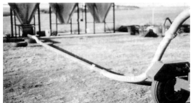
FIGURE 10. Increased Intake Pipe Length.
