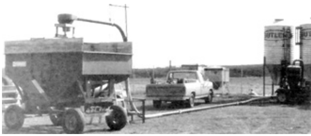
FIGURE 11. Increased Discharge Pipe Length.
