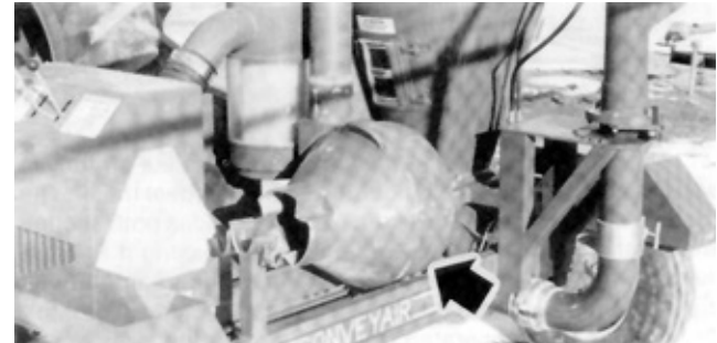
FIGURE 7. Discharge Cyclone Mounted in Transport Saddle.
