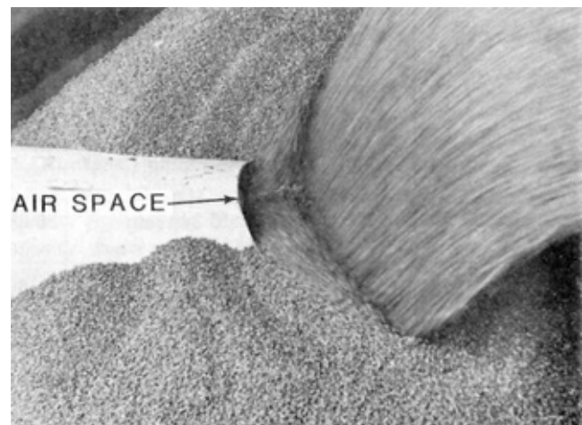
Figure 6. Intake Nozzle showing Air Space Required for Obtaining Maximum Conveying Rates.
