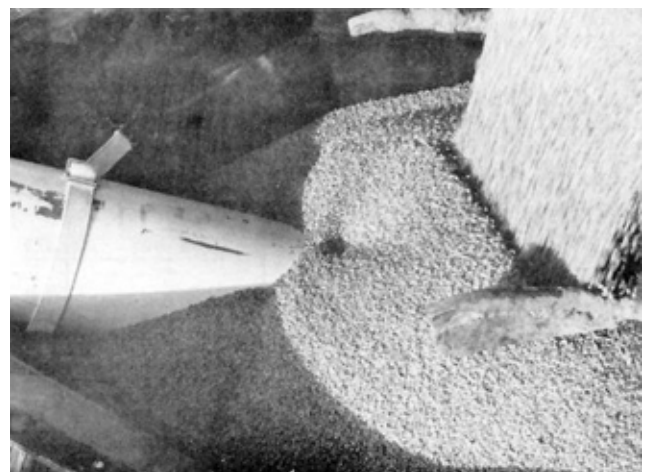
Figure 7. Intake Nozzle Buried in Grain Resulting in Reduced Conveying Rates.
