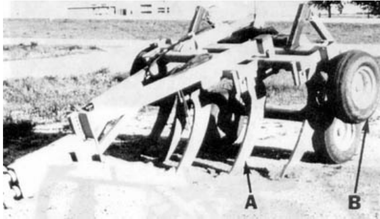
FIGURE 5. Kello-Bilt Series 5000 Subsoiler: (A) Shank, (B) Outrigger Wheels.
