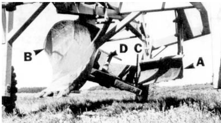
FIGURE 4. Wheel Plow: (A) Grader Blade, (B) Moldboard, (C) Rotating Disc.
