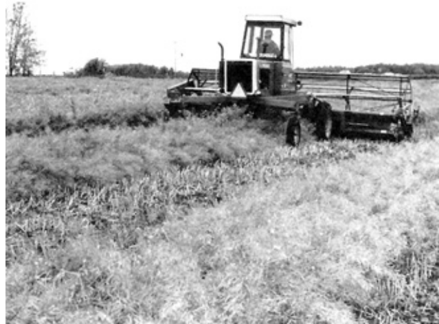
FIGURE 4. Windrowing Rapeseed with the Glendale Attachment.
