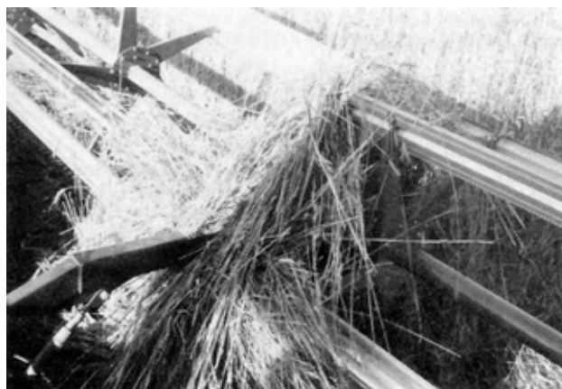
FIGURE 2. Material Caught on the Reel Arm.
