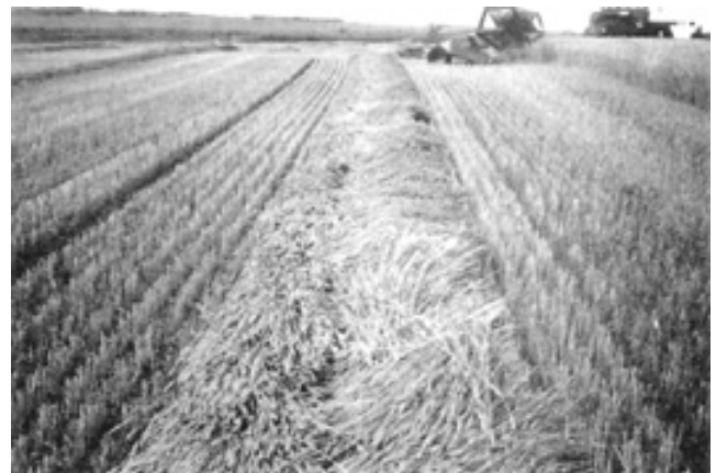
FIGURE 4. Effect of Draper Speed on Windrow Formation: (1) Left side Formed with Normal Draper Speed, (2) Right Side Formed with High Draper Speed.
