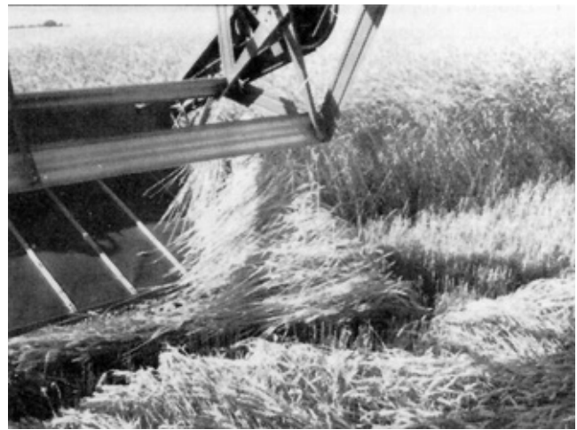
Figure 11. Hairpinning of Cut Stalks on Grain Divider in Leaning Crops.
