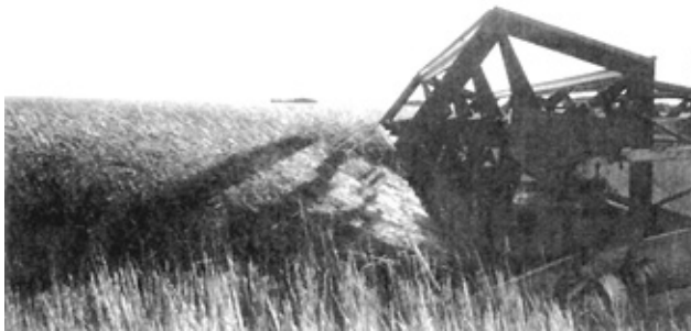
FIGURE 3. Inadequate Forward Reel Positioning.
