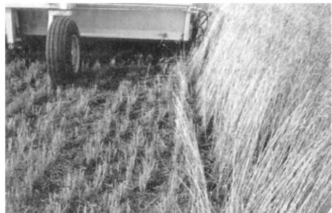
FIGURE 2. Crop Flattened by the Divider.
