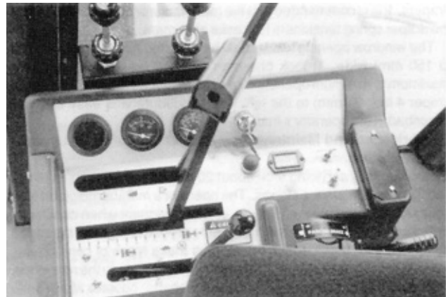
FIGURE 11. Operator Station Instruments and Controls.
