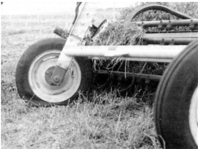
FIGURE 8. Bolt Failure on Reel Basket.
