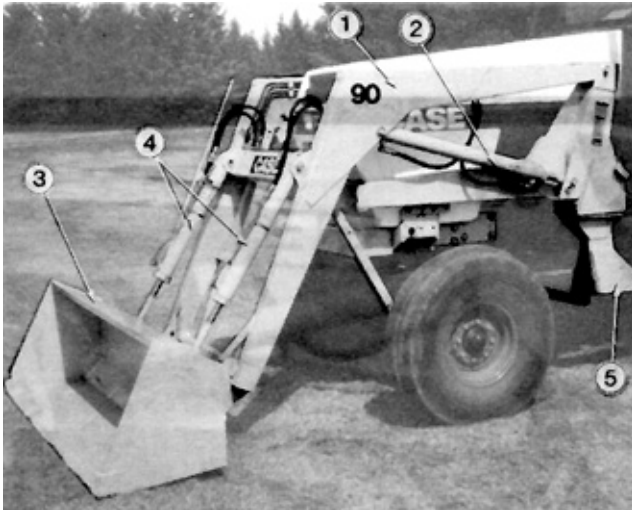
FIGURE 1. Main Components: (1) Lift Arms, (2) Lift Cylinders, (3) 83" Material Bucket, (4) Bucket Cylinders, (5) Tractor Frame Mount.
