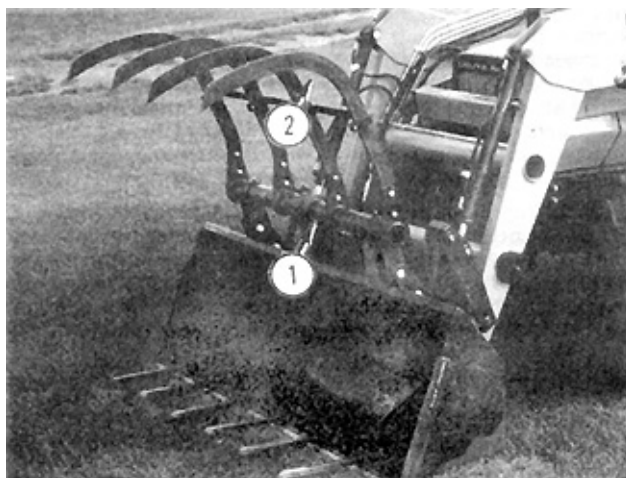
FIGURE 6. (1) Bent Bearing Pillar, (2) Area of Grapple Hook Deformation.
