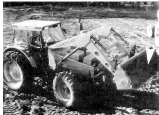
FIGURE 3. Damp Material Adhering to Bucket Walls.
