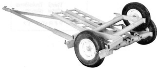
FIGURE 2. Transporter in Folded Position.
