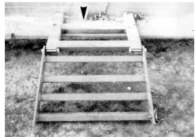
FIGURE 3. Windrower Loading Ramps Showing Spacer Added to Increase Header Clearance.
