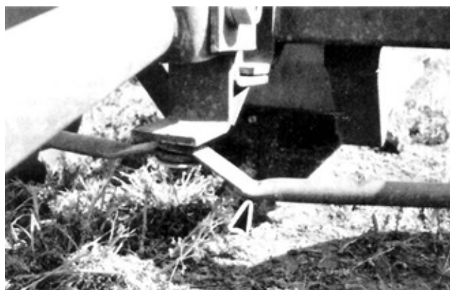
FIGURE 5. Bent Steering Tie Rod.
