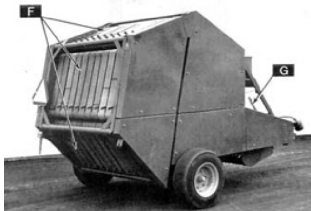
Figure 3. Rear View of McKee 1500 Round Baler. Identification of components: (F) Forming Belts, (G) Pickup Transport Lever.
