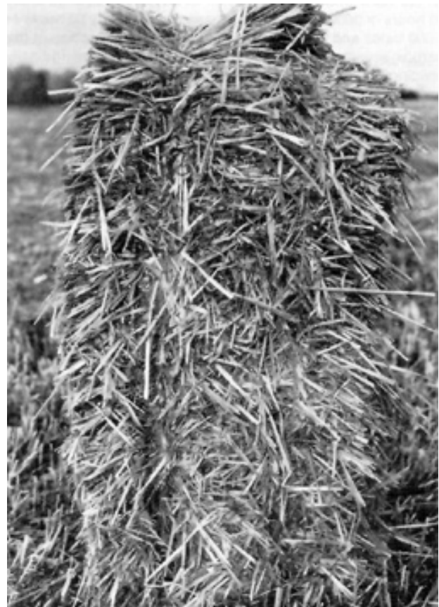
FIGURE 7. Poorly Formed Bale in Greenfeed due to Inadequate Packer Finger Adjustment.
