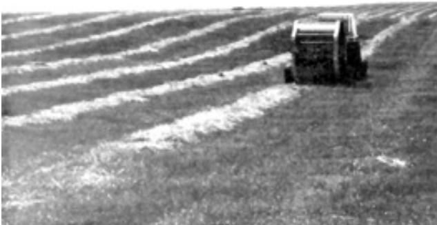
FIGURE 8. Windrow Dropping Out Behind the Baler in Light, Dry Crop Conditions.
