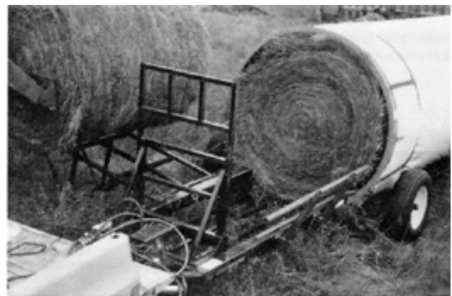
FIGURE 2. Bale from Expanding Chamber Baler being Set onto the Ramp.
