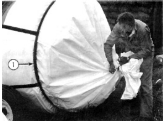
FIGURE 5. Poly Tubing Sleeve End Wrapped and Tied after Installation on Drum; (1) Tension Ring.
