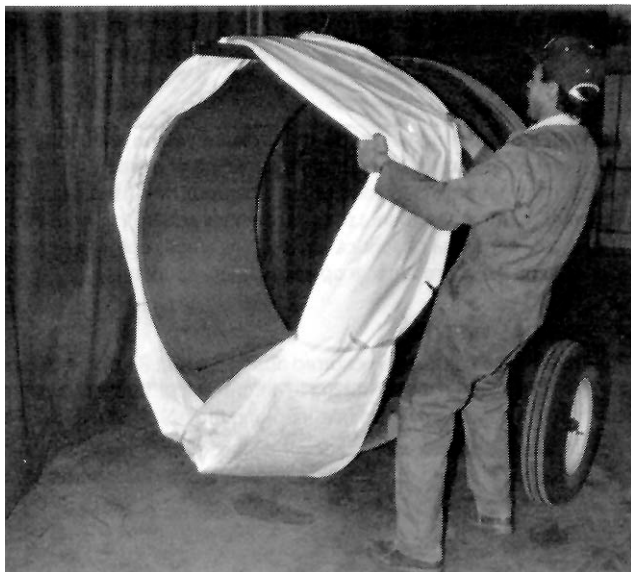
FIGURE 4. Installing Folded Poly Tubing onto the Drum.
