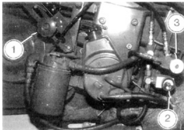
FIGURE 6. Bale Settings: (1) Bale Size Control Knob, (2) Twine Wrap Control Valve, (3) Net Wrap Control Valve.
