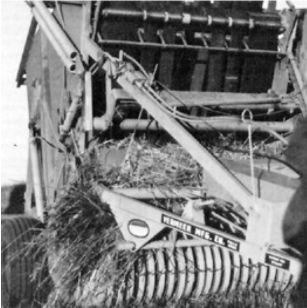
FIGURE 9. Hair-pinning of Long Hay on Baler Side Members.
