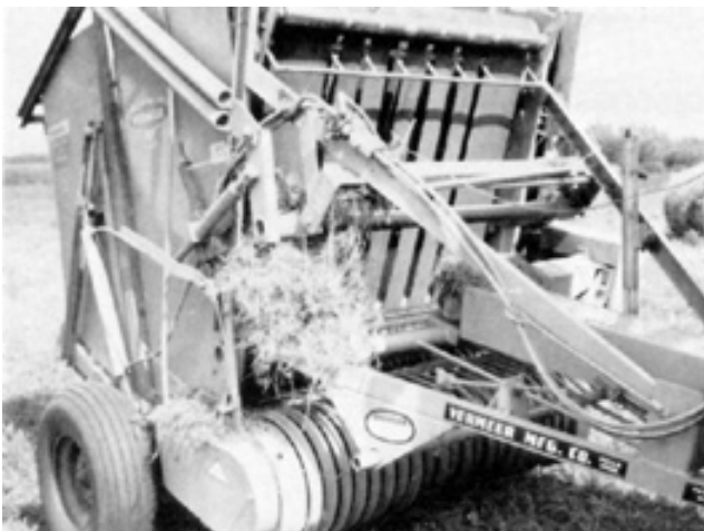
FIGURE 7. Hay Buildup on Twine Wrapping Mechanism.
