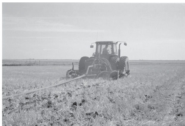
The umbilical injection system at work.
