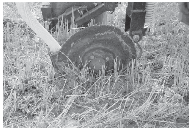
PAMI/Bourgault Low Disturbance Manure Injection Opener.
