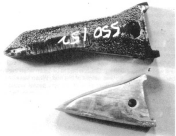
FIGURE 9. Point Wear: Top - New Point, Bottom - Worn Point.
