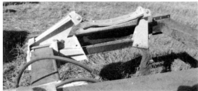
FIGURE 13. Over-Centred Leaf Spring.
