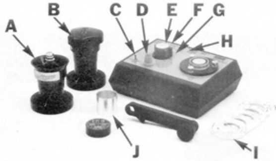
FIGURE 1. Protimeter Grainmini III Moisture Meter: (A) Grinder, (B) Compressor, (C) Switch, (D) Calibration Knob, (E) Meter Dial, (F) Calibrate Light, (G) Meter Scale, (H) Read Light, (I) Reader Rings, (J) Grain Cell.
