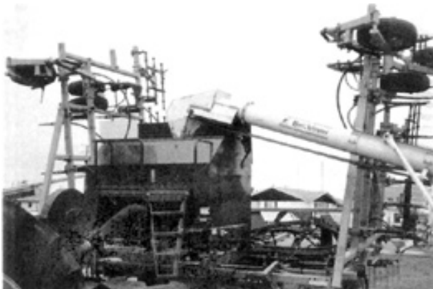
FIGURE 5. Filling with a Conveyor Auger.
