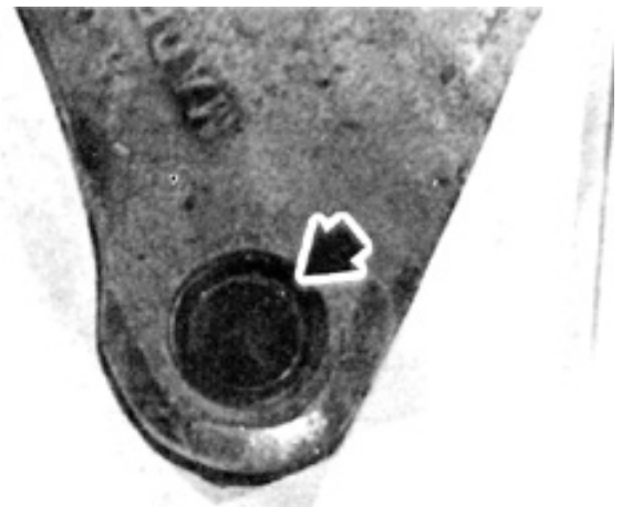
FIGURE 9. Example of Faulty Casting of Double T Slot Adaptor.
