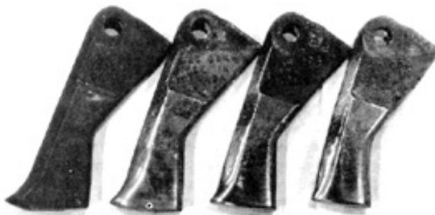
FIGURE 7. Wear on the Banding Blades After 13 ac (5.2 ha) per Blade, 20 ac (8 ha) per Blade and at the End of the Test.
