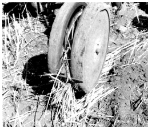
FIGURE 7. Trash Trapped Between Packers at Narrow Spacing.
