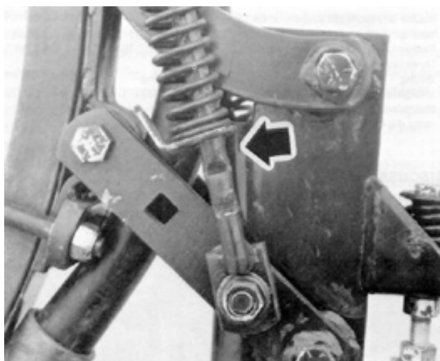
FIGURE 9. Spring Tension Adjustment for Packing Force.
