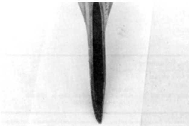
FIGURE 17. Wear on the Fertilizer Boot.
