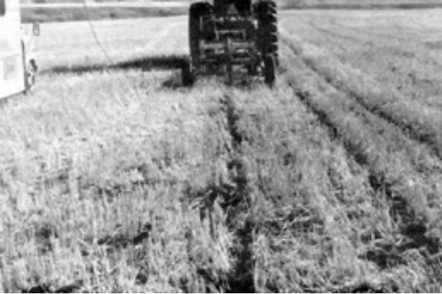
FIGURE 2. Soil Disturbance and Soil Opening (Upper: Conventional Cultivator Chisel Point; Lower: Typical Banding Knife).
