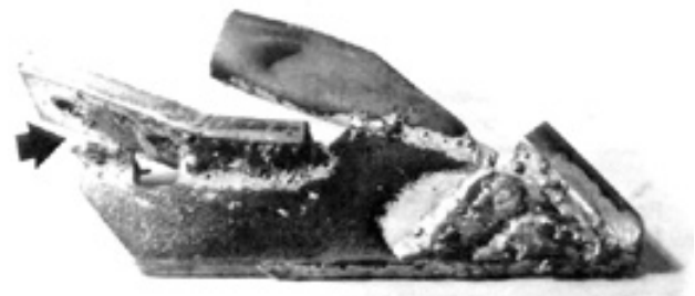
FIGURE 18. Broken Support Bracket.
