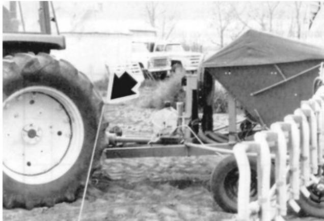
FIGURE 8. Disc Marker Cable and Tractor Tire Interference.
