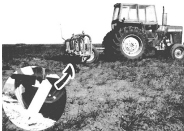
FIGURE 7. Tilting Frame Necessitating Rear Wheel Removal when Attached to Tractors with High Drawbars
