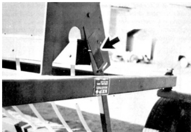
FIGURE 10. Metering Shaft Indicator Fabricated by PAMI.
