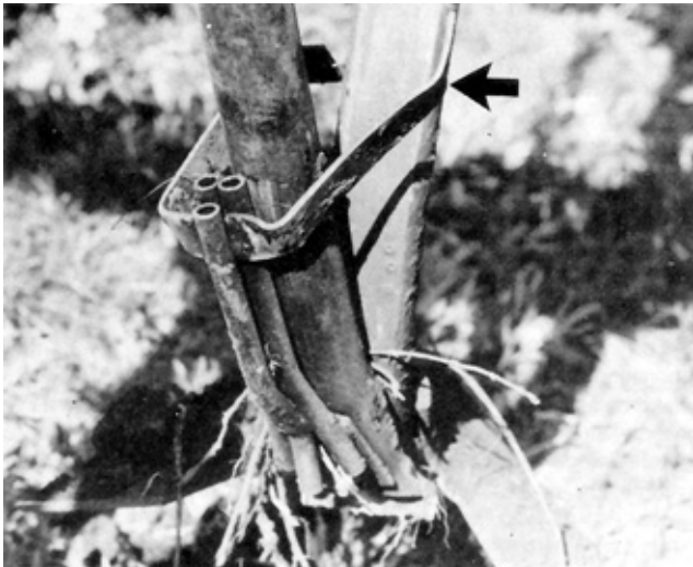
FIGURE 19. Damaged Seed Boot Clamps.
