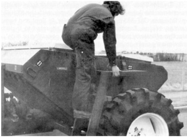
FIGURE 19. Tank Access Ladder.
