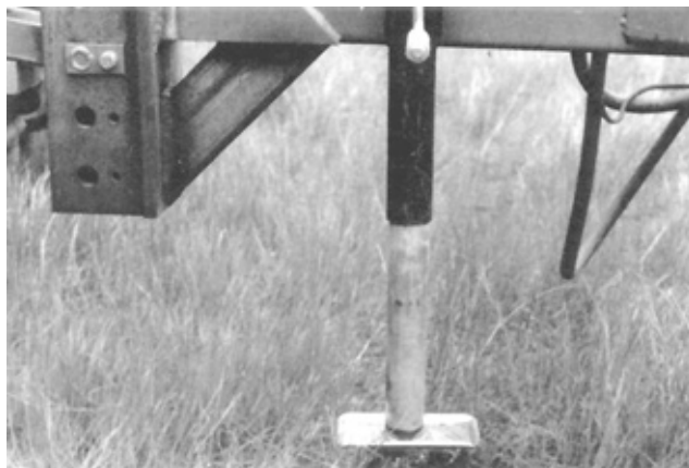
FIGURE 17. Inadequate Lifting Height of Hitch Jack.
