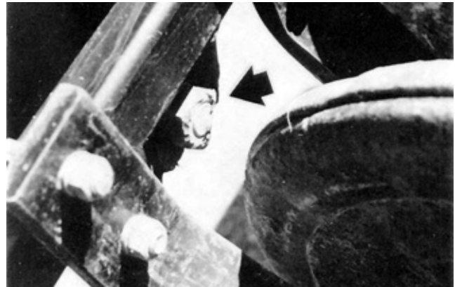
FIGURE 14. Bolt Wear on Gang Pivot Point.
