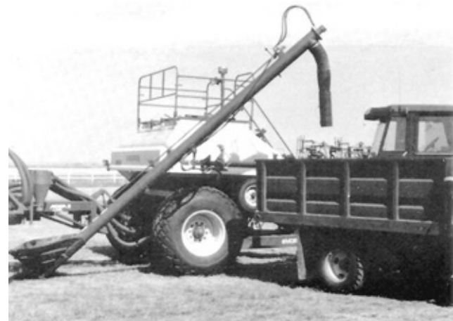
FIGURE 15. Using Clean-Out System.
