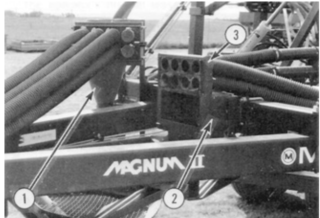
FIGURE 14. (1) Cyclone, (2) Sample Collector, (3) Air Seeder Distribution.
