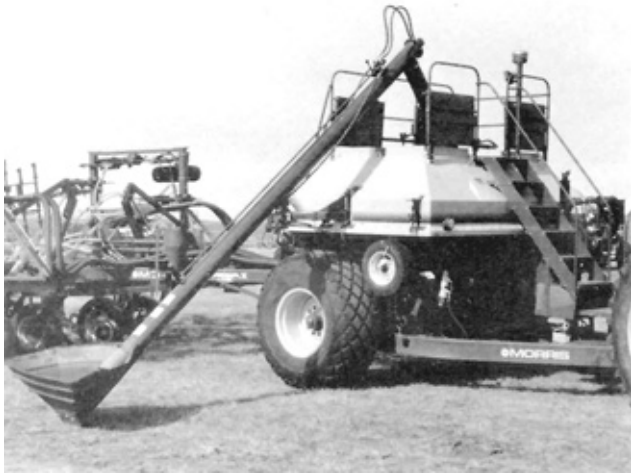
FIGURE 12. Fill Position of Auger.
