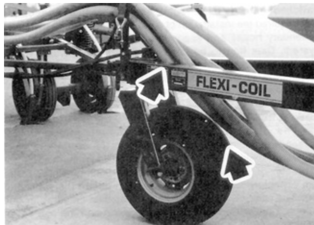
FIGURE 21. Interference at Front Pivot Point.
