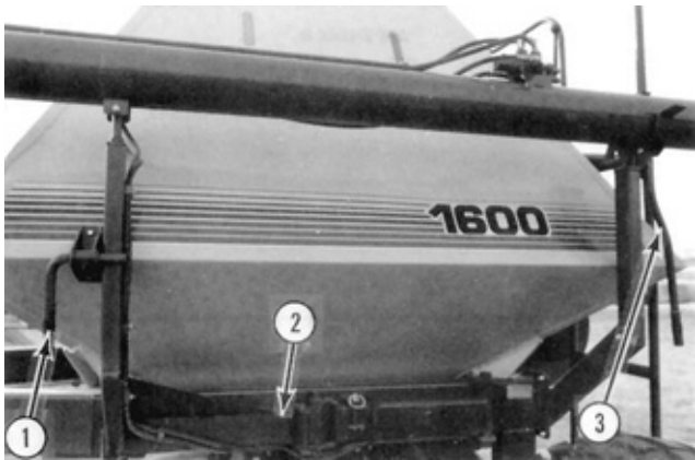
FIGURE 14. Auger in Transport Position: (1) Front Lock Arm, (2) Front Pivot Arm, (3)Rear Lock Handle.
