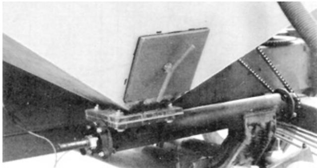
FIGURE 18. Tank Cleanout Door.
