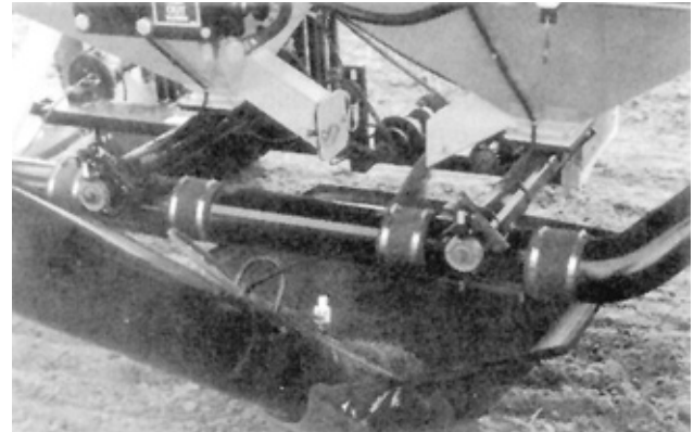
FIGURE 20. Unloading Material From Bourgault Tank.
