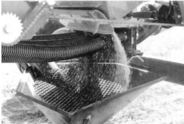
FIGURE 14. Unloading Material from Morris Tank.
