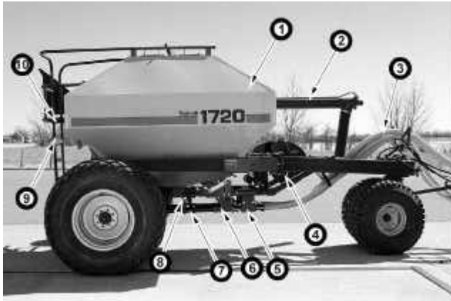
Figure 1. Flexi-coil 1720 Air Cart: (1) Tank, (2) Auger, (3) Primary Hose, (4) Centrifugal Fan, (5) Centre Manifold, (6) Metering Drive System, (7) Intermediate Manifold, (8) Hand Crank, (9) Ladder and (10) Rear Platform.
