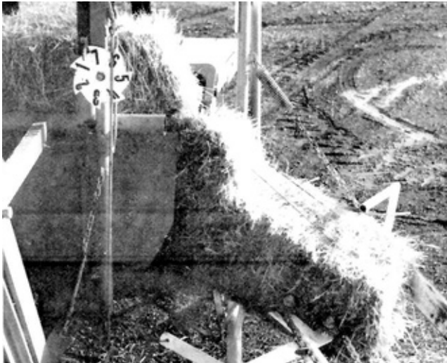
FIGURE 9. Loose Bale Wedged on Bale Chamber Side.
