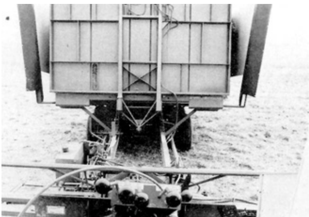
FIGURE 9. Limited Visibility when Backing into the Stack.
