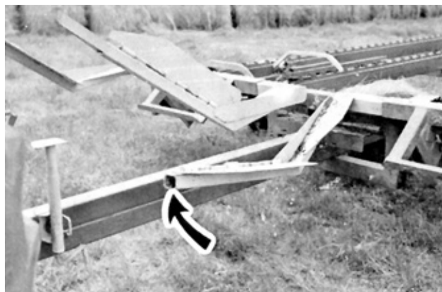
Figure 10. Broken Tip on Pickup Fork Tine.
