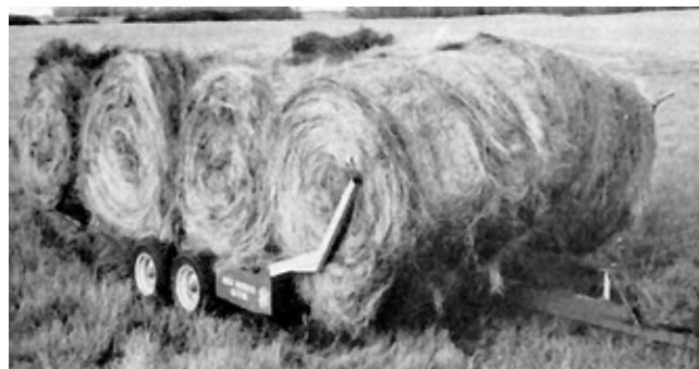
Figure 5. B & K 815 Fully Loaded in Transport Position.
