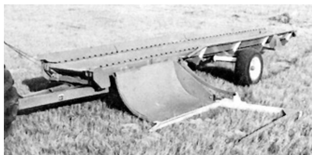
Figure 2. McKee Bale-rustler in Loading Position.
