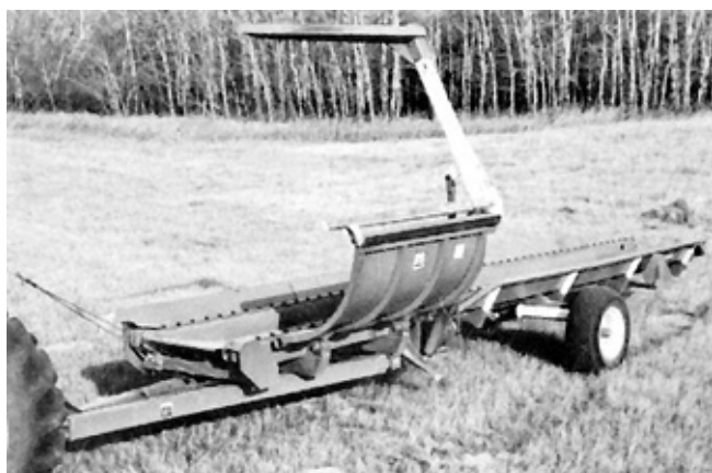
Figure 1. McKee Bale-rustler in Transport Position.
