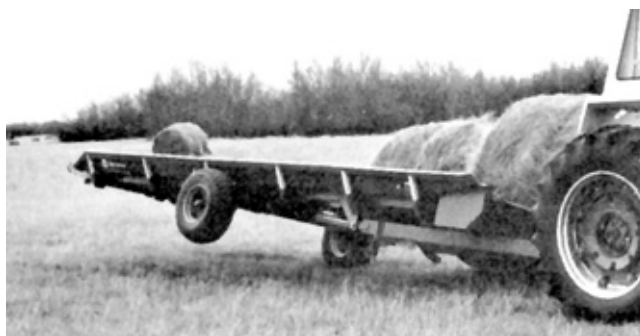
Figure 3. Sideways Tipping of the Bale-rustler when the First Bale Loaded Weighs More than 680 kg (1500 lb)
